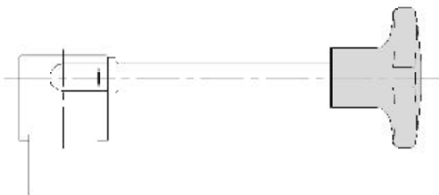
Fig. 7. LKB butterfly valve regulating handle
