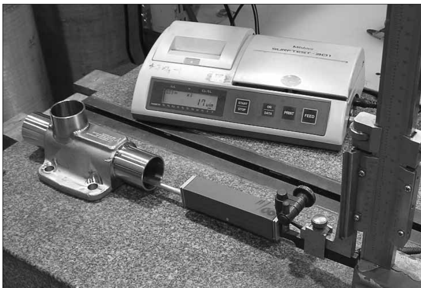
Profilometer Check for Valve Surface Finish
