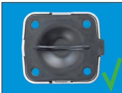
6. Then turn the diaphragm (with 2-piece diaphragms only the PTFE face) back anti-clockwise to the next possible bolt alignment (max. 180°). Ensure that the compressor, the sealing weir and the diaphragm are aligned (return the PTFE face to its original shape).
