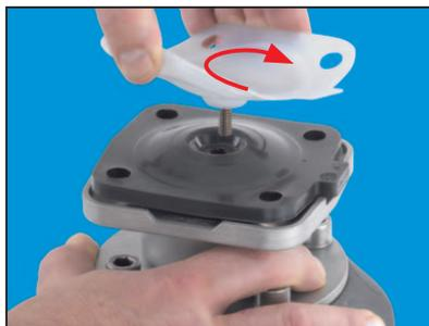
5. Screw new diaphragm into spindle / compressor until you feel strong resistance. With 2-piece diaphragms place the elastomer backing onto the actuator / bonnet flange so that it fits perfectly, invert the PTFE face and proceed as described above.
