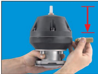
3. Move the actuator / bonnet to the „closed“ position. For manual bonnets make sure that it is only closed so far that the compressor stays in its outer guides.
